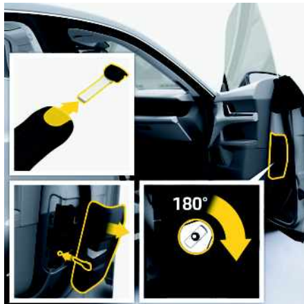
Fig. 44: Performing emergency locking of the passenger's door
