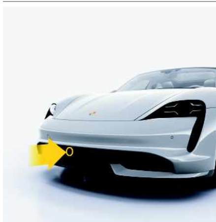
Fig. 7: Location of the radar sensor
