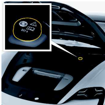
Fig. 35: Brake fluid reservoir
