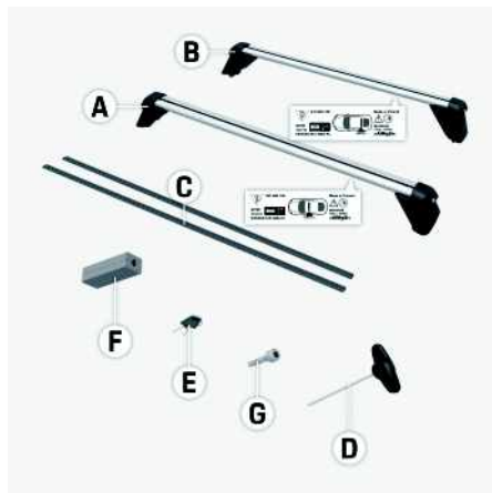
Fig. 160: Components of the roof transport system
