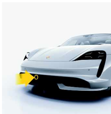
Fig. 145: Location of the radar sensor
