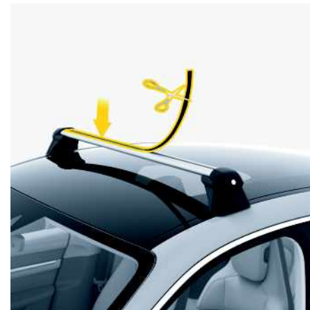
Fig. 174: Cutting the profile trims to size and attaching
