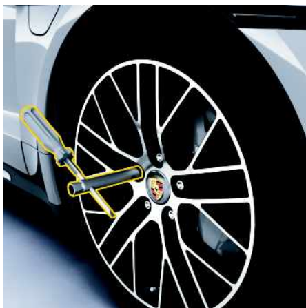
Fig. 215: Screw in one assembly aid on vehicles without PCCB
