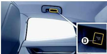
Fig. 93: Operating reading lights
