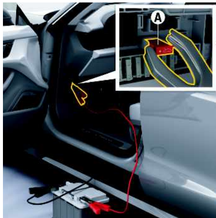
Fig. 33: Emergency unlocking of the bonnet – connect positive pole
