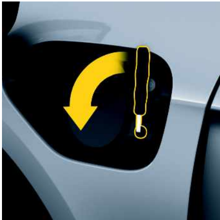
Fig. 54: Emergency release of the manual charge port door
