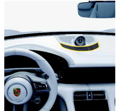
Fig. 21: Upper ventilation panel
