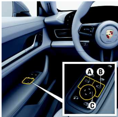
Fig. 125: Swivelling down mirror glass as a parking aid
