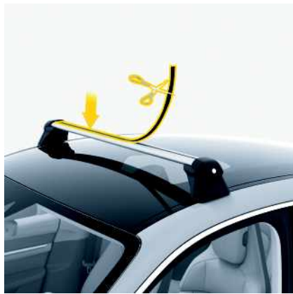
Fig. 172: Cutting the profile trims to size and attaching
