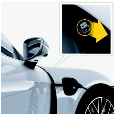
Fig. 56: Performing an emergency release of the vehicle plug
