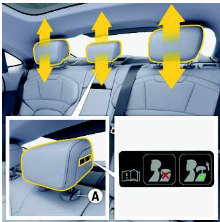
Fig. 184: Setting the height of the headrests on the rear seats (example: 3 rear seats)
