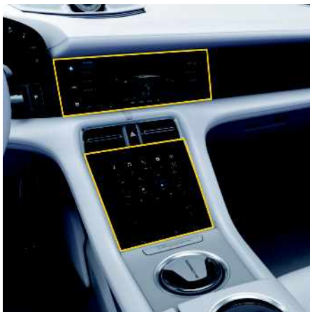
Fig. 5: Air-conditioning control panels
