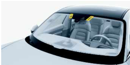
Fig. 129: Attaching toll devices
