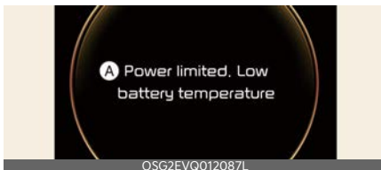
A: Power limited. Low battery temperature
