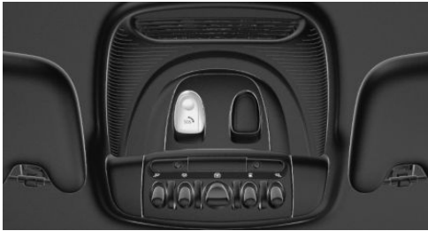
SOS button in the roofliner
