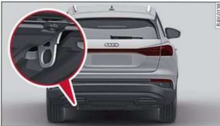
Fig. 168 Rear of the vehicle: towing eye for professional towing services
