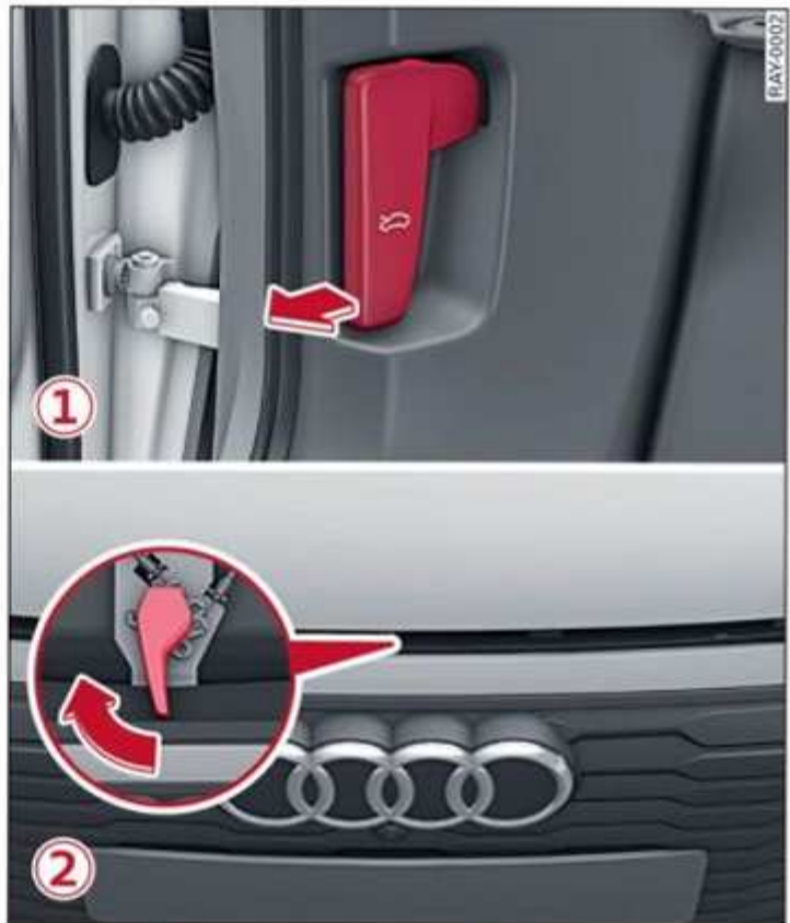
Fig. 149 ① Footwell: release lever; ② front compartment: lever to open the hood
