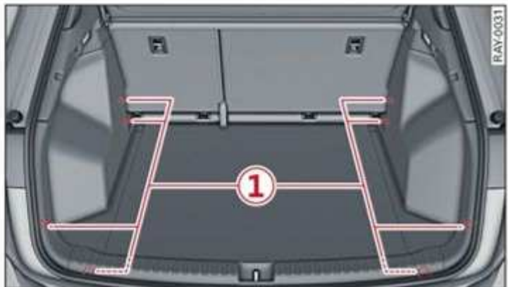
Fig. 72 Luggage compartment: location of the tie-downs
