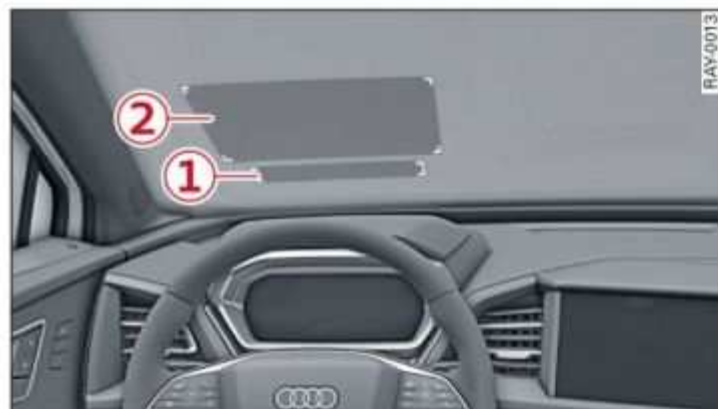
Fig. 19 Windshield: display areas of the head-up display
