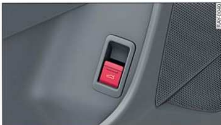
Applies to: vehicles with automatic luggage compartment lid: Fig. 30 Driver's door: opening the luggage compartment lid
