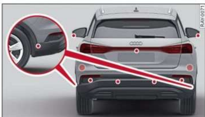
Fig. 95 Rear area: sensors and cameras
