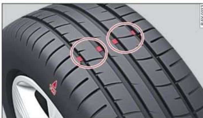
Fig. 157 Tire profile: treadwear indicator
