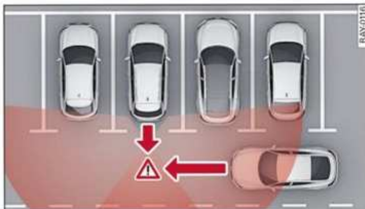
Fig. 126 Sensor detection range for rear cross-traffic assist
