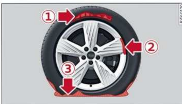
Fig. 161 Tire: tire damage that cannot be repaired
