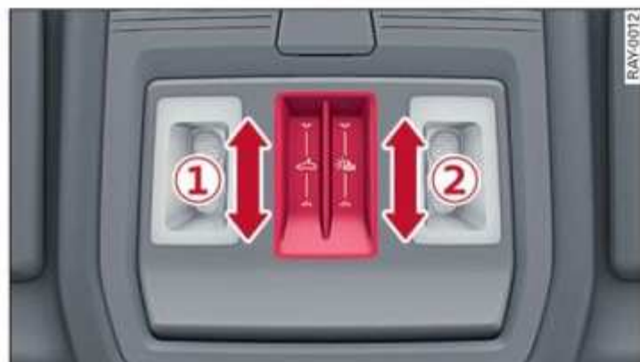
Fig. 36 Headliner: controls for the panoramic glass roof ①, the roof ②, and for the sunshade
