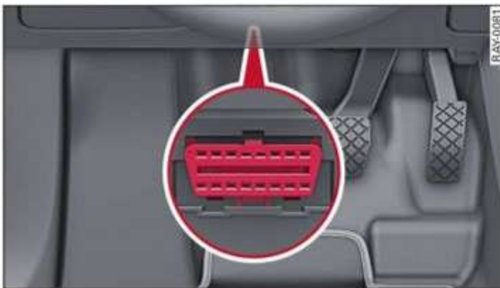
Fig. 175 Driver's side footwell: connection port for the On Board Diagnostic System (OBD)
