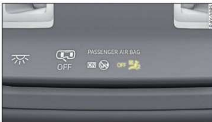
Fig. 63 Headliner: indicator light to display the status of the front passenger's airbag
