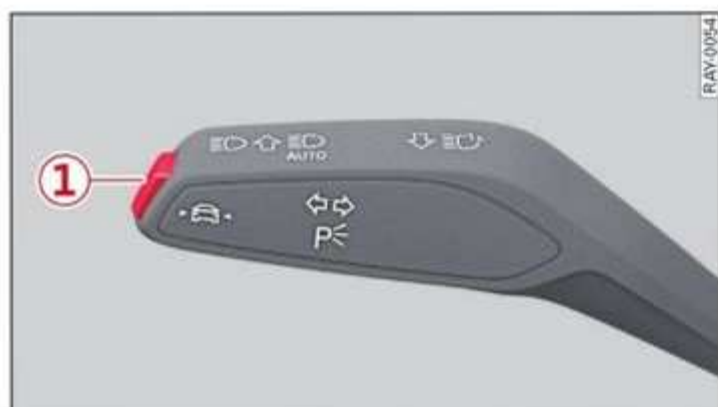
Fig. 115 Turn signal lever: button for lane departure warning and lane guidance for adaptive cruise assist*
