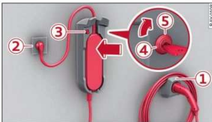
Fig. 90 Wall mount clip: securing the Audi charging system
