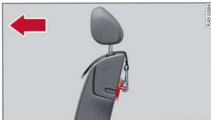
Fig. 66 Rear backrest: securing the upper belt to the top tether anchor
