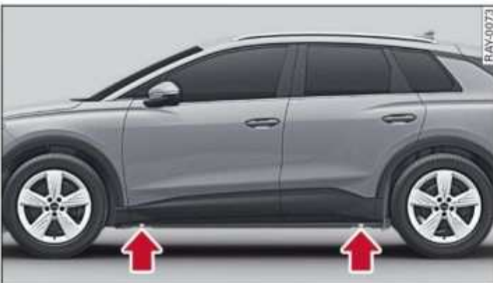
Fig. 165 Sill panels: markings
