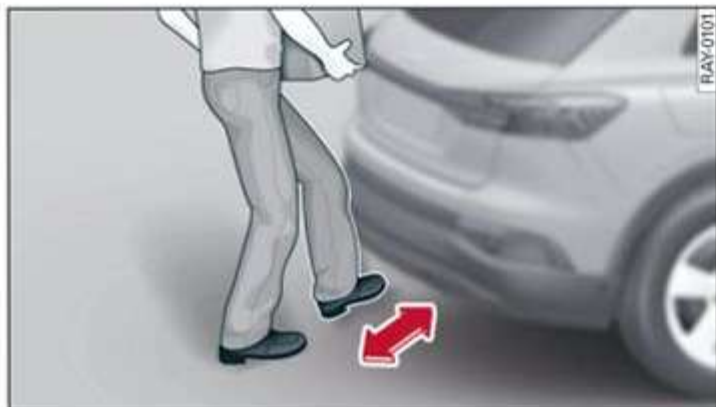
Fig. 32 Vehicle rear: foot motion (example)
