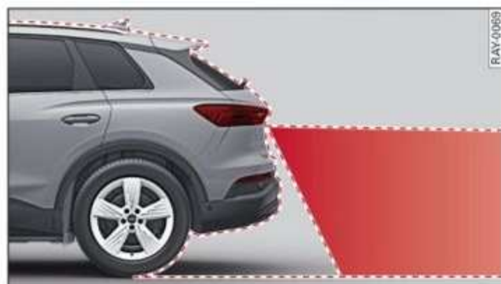
Fig. 93 Rearview camera coverage area
