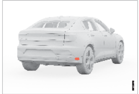
Location of rear radar units
