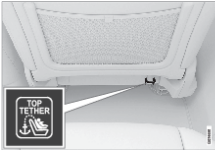
The mounting point location for the front seat is indicated by a symbol on the rear of the front seat.
