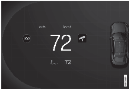
Examples of information on speed camera and speed limit in the driver display
