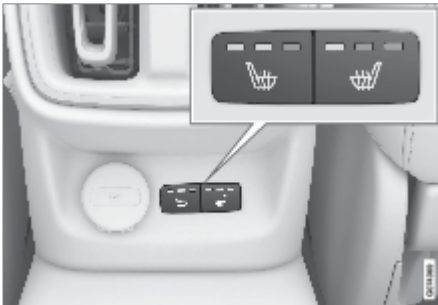
Buttons for heated rear seats on the tunnel console.
