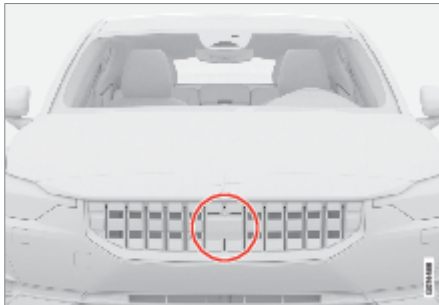
Location of front radar units
