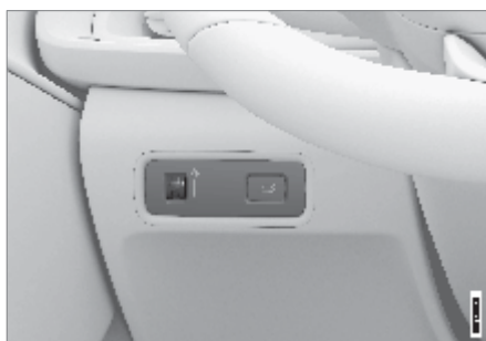
Thumbwheel (to left) for adjusting interior brightness.
