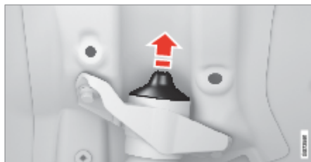
The rubber cover is positioned on top of the adjusting knob.
