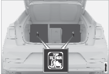
Mounting point locations for the rear seat are indicated by symbols on the rear of the backrest.
