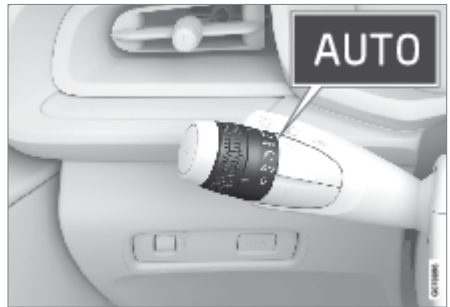
Stalk switch rotating ring in AUTO position.
