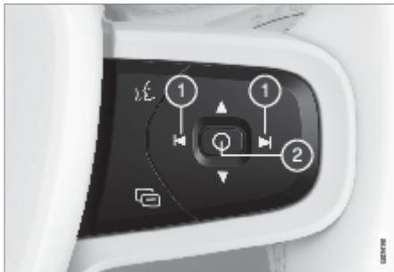
Right-hand keypad on the steering wheel.
