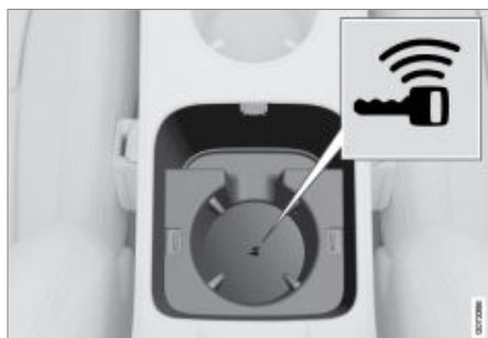
Backup reader's location in the tunnel console.
