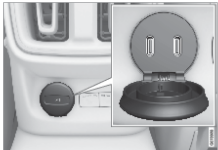
USB ports (type C) in tunnel console, rear seat.
