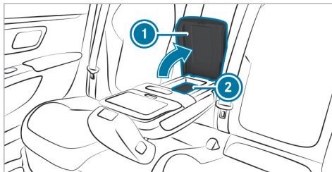
Wireless charging in the rear passenger compartment in vehicles with MBUX rear tablet
