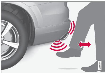
Kicking motion within the sensor's activation area.
