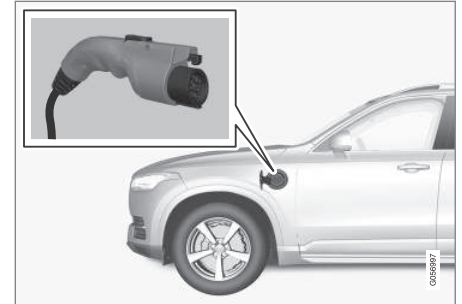
Charging cable handle and charging socket.
