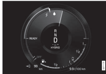
The instrument panel gauge when both the electric motor and the combustion engine are being used.
