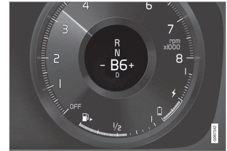
Gear shift indicator in the driver display 5 .
